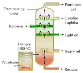
Fractional distillation of petroleum
